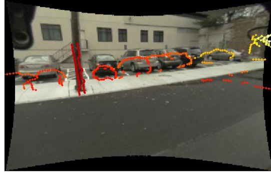
Figure 7. Example alignment of Cam2 using the reprojection / reconstruction technique of Sec. 6 but before discontinuity matching. The rotation and field of view are getting close, but more refinement is necessary to make use of the fused data. For illustration purposes, only the depth-discontinuous lidar locations are shown. This technique is described in Sec. 7
